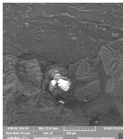
Fig. 7. SEM analysis - light spherical particles - oxides and exposed dendrites on the fracture surface
